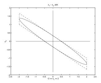
Figure 4: The Stability Region (Solid Line) of the Closed-Loop Plant in Example 4.1 with Control Law  $u = -2x_1 - 3x_2$
