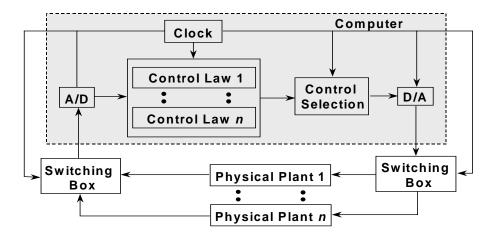
Figure 1: A Typical Real-Time Computer-Controlled System
