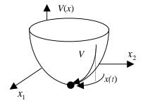
Figure 3.b Illustration of a Lyapunov function.
