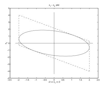
Figure 5: The Stability Region (Solid Line) for the Designed Safety Controller in Example 4.2
