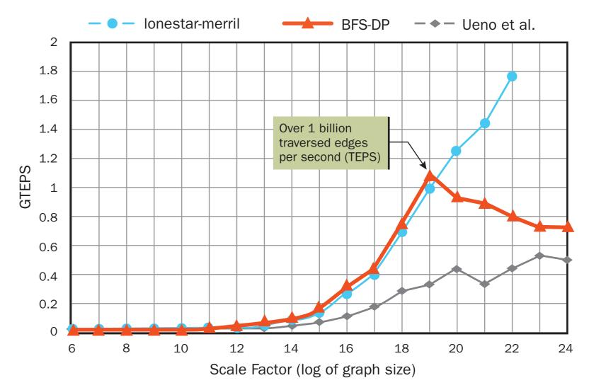
BFS performance reported by P. Zhang, et al.,, "Dynamic Parallelism for Simple and Efficient GPU Graph Algorithms," submitted to 5th IEEE Workshop on Irregular Applications: Architectures and Algorithms, Nov 2015.
