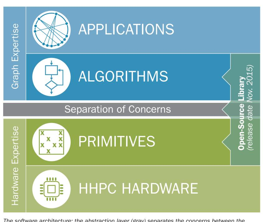
The software architecture: the abstraction layer (gray) separates the concerns between the expertise needed to develop graph algorithms and applications (above), and intimate knowledge of the hardware needed for high performance (below).
